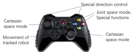
Fig. 1. Function assignment for the joystick.
