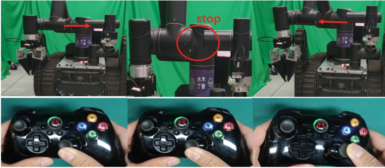
Fig. 11. The process of the longer arm approaching the object easy to collide (Color figure online)
